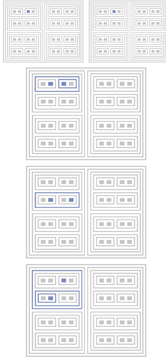
Figure 5: Visual illustration of addition: FC\left(\frac{59}{12}\right) + FC\left(\frac{49}{24}\right) . The uppermost illustration displays the N_{FC} block, which remains unchanged. The second uppermost illustration shows R_{FC} block arithmetic, which takes \tau(\chi_{(2,-,-)}(\frac{59}{12})) = (0, 1) as input and yields \tau(\chi_{(2,-,-)}(\frac{167}{24})) = (1, 0) as output, whose register is separated by two hops. The middle illustration displays the L_{FC} block arithmetic, which takes \tau(\chi_{(-,3,-)}(\frac{59}{12})) = (1, 0, 1) as input and yields \tau(\chi_{(-,4,-)}(\frac{167}{24})) = (1, 1, 1) as output, whose register is separated by one hop. The lowermost illustration displays the T_{FC} portion arithmetic, which takes \chi_{(-,-,2)}(\frac{59}{12}) = (0, 1) as input and yields \chi_{(-,-,3)}(\frac{167}{24}) = (1, 0, 1) as output, whose register is separated by three hops.
